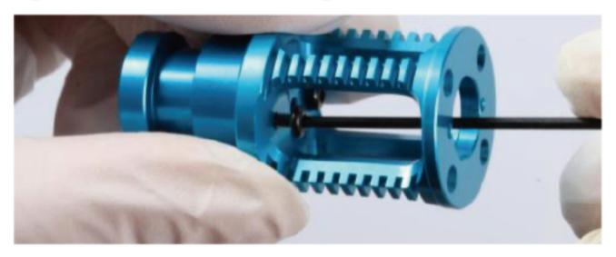
2. Screw the heatbreak into side A of the heatblock with the 7.8mm open – ended wrench using strength about 4.5nm.
