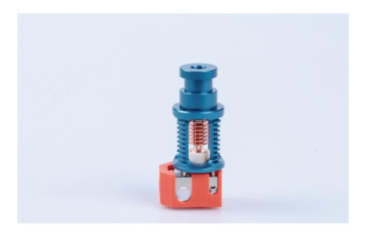
7. If you are using glass ball type thermocouple, put the thermocouple into the brass sleeve in the attachment first (the brass sleeve is shown in the figure below), and the port should be sealed with the heat conducting silicone grease carried in the attachment, and then put it into the heatblock and lock them with the head screw.
