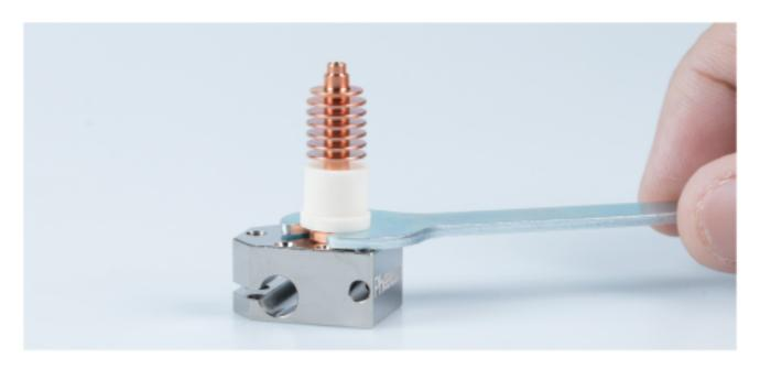
3. Carefully align the 4 supporting tubes of the heatsink with the 4 holes on the side A of the heatblock, press them tightly. Meanwhile, please note that the top of the heatbreak should be completely close to the holes on the top of the heatsink. If not properly aligned, heatbreak could be damaged during hot – tightening.
