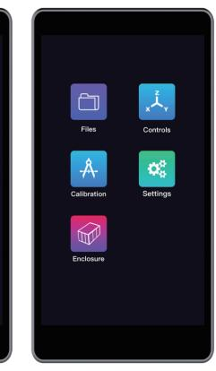
When the machine is under working condition, you can swipe left on the Touchscreen to control the LED Strips and the Exhaust Fan.
