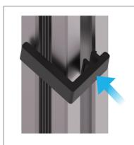
Tilt the snap joint of the Cable Clip and press it against the groove of the beam to clip it in. The sheet of the Cable Clip should hold the cable inside the adjacent groove.
