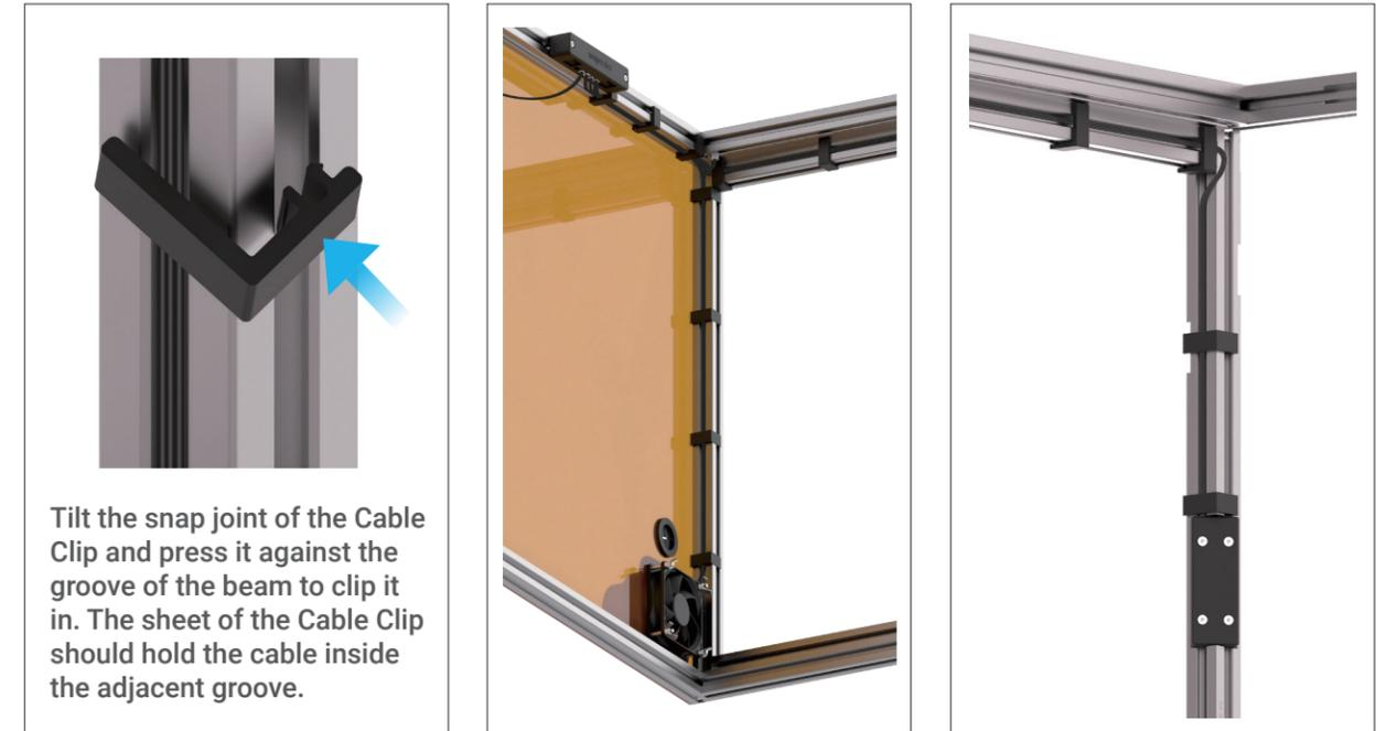
Tilt the snap joint of the Cable Clip and press it against the groove of the beam to clip it in. The sheet of the Cable Clip should hold the cable inside the adjacent groove.
