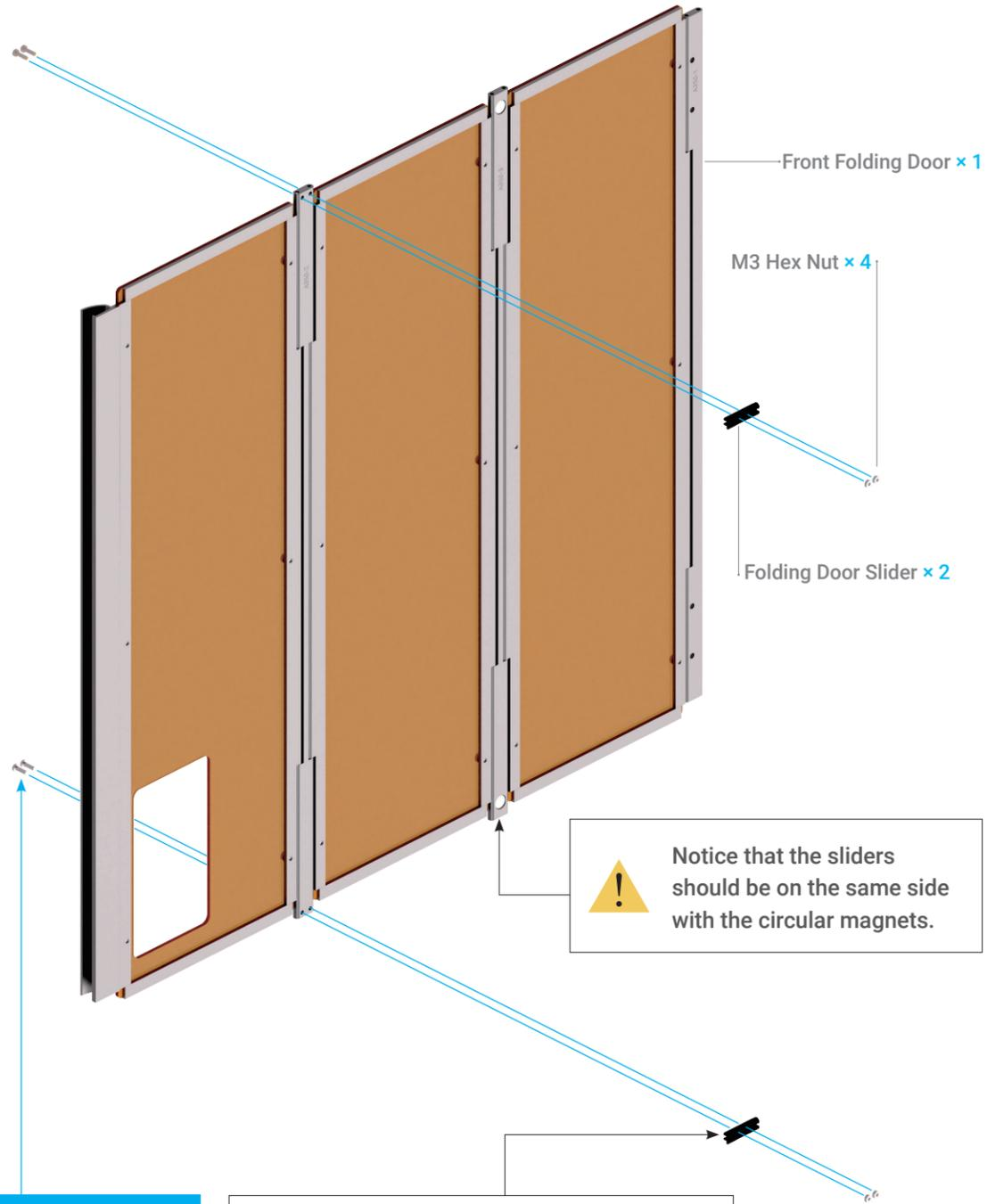
**!** Notice that the sliders should be on the same side with the circular magnets.
