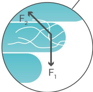
$F_1 = f(\text{mass, } 1/\text{rigidity of the polymer}) = f(\text{layer height, overhang angle, temp.})$
