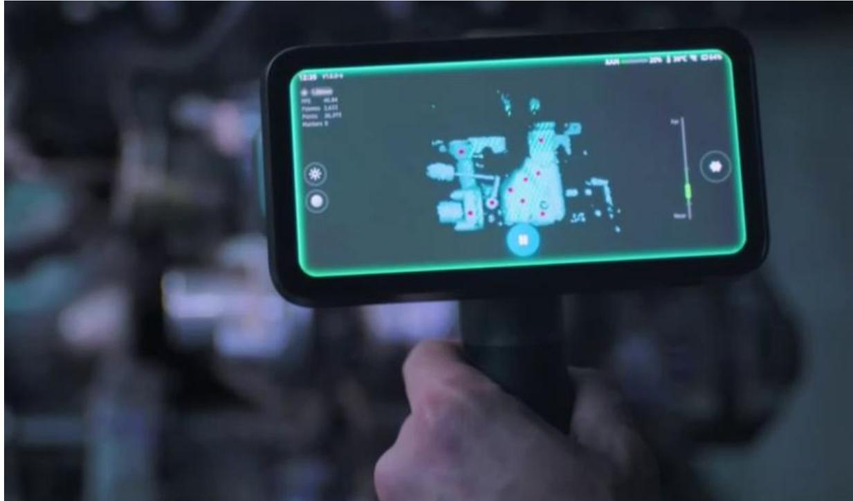
**7** parallel laser lines can obtain **better data quality and details**. On the contrary, this will require longer scanning time and only be practicle for small range.
