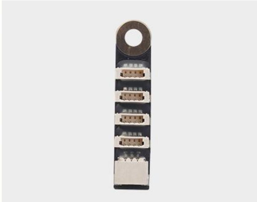
The WS2812 LED Hub is used to connect the LEDs supporting WS2812 protocol to the WS2812 Port on the RC receiver shield, thus enabling independent control of more LEDs. It is suitable for all kinds of models that need to use multiple LEDs.
