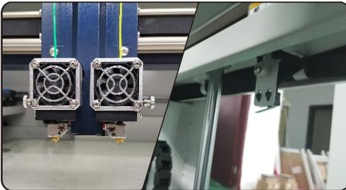
If the nozzle can't touch the platform even loosen all the leveling nut, you can move Z stop limit a little up, as you can see from figure.
