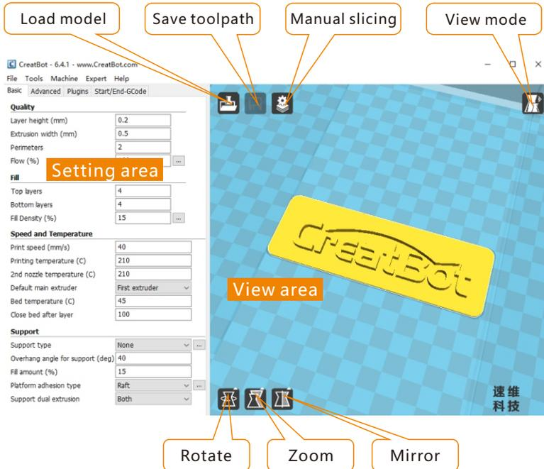
As you can see from the complete UI, the left side of the software is setting area, the right side is view area. The setting area contain "Basic", "Advanced", "Plugins", "Start/End GCode" four tabs. The Basic tab is the most common settings, usually the most frequently used parameters are here. Each parameter has a mouse-over tips, you can set parameters according the prompt. If you want to restore the default settings, please click on the menu "Tools"-> "Restore Default".
