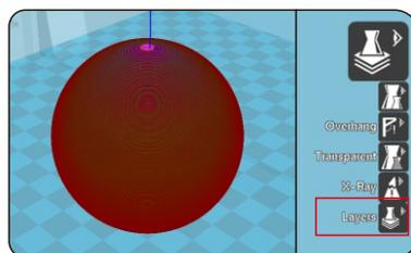
By slice view can easily observe the generated path, you can easily observe the different layers of sliced by slicing altitude indicator, use Ctrl + arrow keys can also be observed layer-by-layer.
