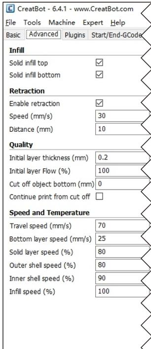
**Solid fill top:** Refers to whether to print the top surface of the model, uncheck will print it with infill method.
