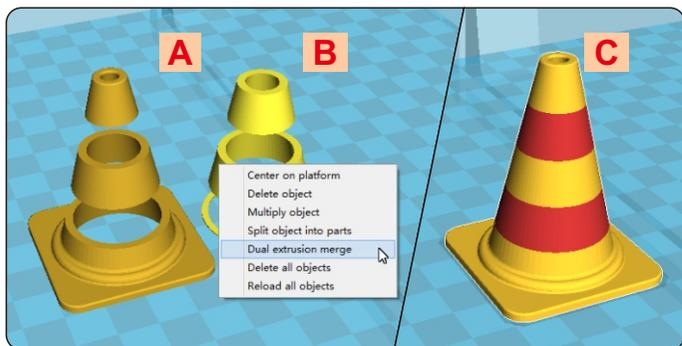
**Step 1:** Load 2 models you want as shown in figure [A] and [B].
