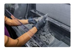
5. Cleanup: After extracting parts, begin cleanup. Powder that accumulates within the workspace can be wiped into the sifter and recaptured for later use. Smaller deposits around the workspace, within the build chamber enclosure, and on the hood can be picked up with the integrated vacuum hose for later disposal. The vacuum is controlled by a physical button conveniently located on the control panel.
