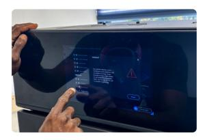
5. Start the print: Once all preprint checks have been completed, the Fuse 1 is ready to print. The home screen transitions to display a live stream of the print bed so you can watch each new layer take shape. This camera view is also available in PreForm.
