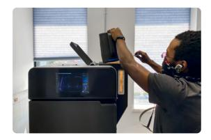
2. Insert a clean optical cassette: Removal, maintenance, and reinstallation of the optical cassette do not require any tools or disassembly. A second cassette enables you to run another print without cleaning one used for a previous print.
