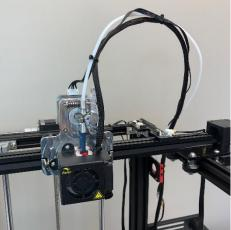
Secure the cables and filament guide tube with zip ties
