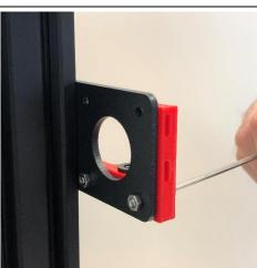
Install the filament guide bracket using provided M3 bolts and nuts
