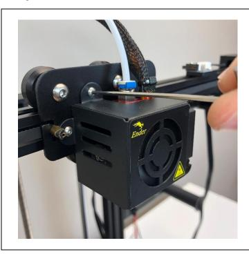
Use the 2mm Allen wrench to remove the fan shroud
