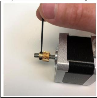
Remove the extruder gear using the 1.5mm Allen wrench
