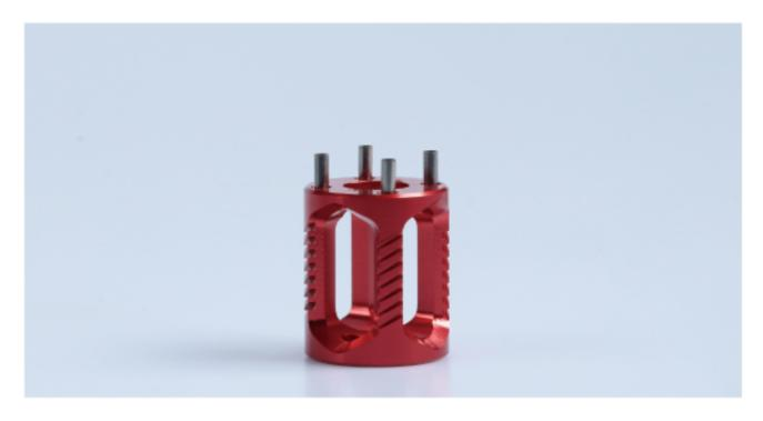
3. Carefully align the 4 supporting tubes of the heatsink with the 4 holes on the A side of heatblock, press them completely. Meanwhile, please note that the top of the heatbreak should be completely close to the holes on the top of the heatsink. If not properly aligned, heatbreak would be damaged during hot - tightening.
