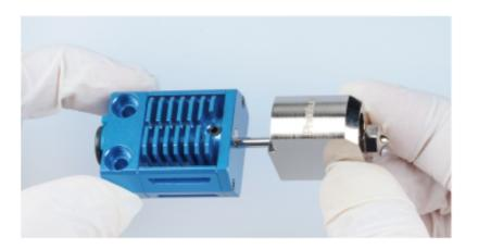
6.Use the H1.5 hexagonal bar to lock the flat head screw M3.0\*4.0 on the front of the heat sink.
