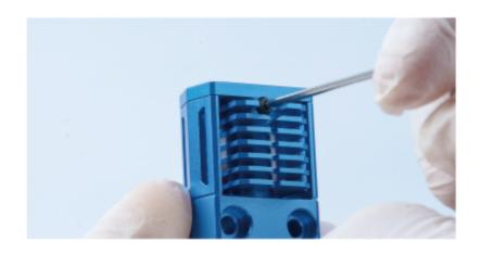
4.Screw the nozzle to the heat block with the H7.0 open wrench. Please note that the hexagonal surface of the nozzle should be tightly attached to the bottom surface of the heat block, and the tightening torque of the nozzle is 2.5NM.
