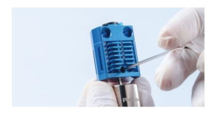
7.On the A side of the heat block, screw 3 flat head screws M3.0\*3.0 into the 3 threaded holes respectively with the H1.5 hexagonal bar.
