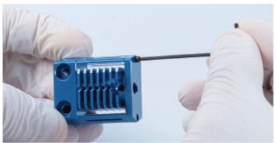
2. Embed the bowden collect into the top of the assembled heat sink, then insert the collect clip in between the bowden collect and the heat sink to fix the bowden collect.
