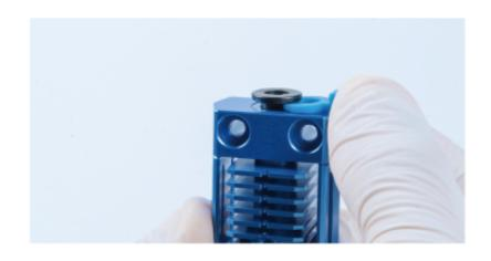
3. Assemble the plunger into the larger hole at the bottom of the heat sink, and screw the flat head screw M3.0\*4.0 into the threaded hole on the heat sink with the H1.5 hexagonal bar (no need to locking), so that the plunger won't fall off. Please note that the hole on the plunger should be directly opposite to the threaded hole on the front of the heat sink, which would ensure that the screw can be smoothly screwed in.
