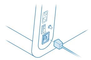
7 Connect the power cable to the machine and an outlet.
