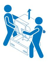
3 Use the cardboard slings to lift the machine off of the base.
