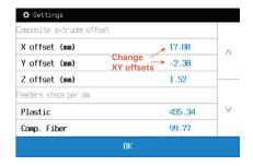
After adjusting the offsets, reprint the offset test and make sure that composite fiber is properly centered(as on the Reference scheme) for both X and Y zero rectangles.
