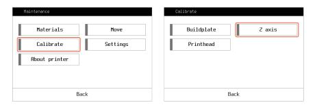
Press Maintenance > Calibrate > Z axis and follow the instructions. You will be asked to use a thin paper sheet to fine tune the gap between the nozzle tip and the buildplate.
