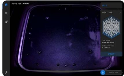
Tap the printer icon in the left sidebar to access the printer status screen. Readouts of the bed temperature, hopper level, powder type, and available credits can be found here.
