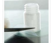
In cases of excess adhesion, it is recommended to wet print bed with a small amount of water slowly working it below the part. This should make part removal easier.
